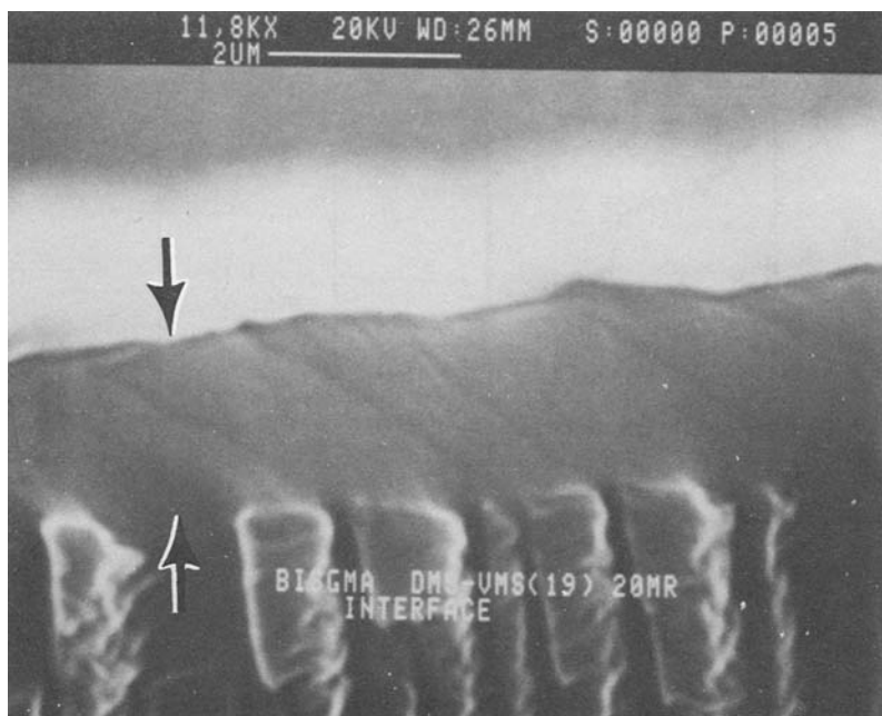
Fig. 8. Scanning electron micrograph showing the thickness (see the region indicated between the arrows) of DMS-VMS (MW 28,000, 19% VMS) gel coating (20 Mrads) on bis-GMA.
